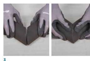
Lightly press the components together to position them. Press the seams together again for final fixing.
