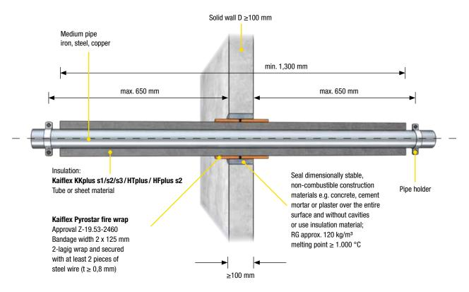
Depending on the installation situation, a Kaiflex Pyrostar fire wrap with a width of at least 125 mm must be installed approx. 70 mm deeply on top of the insulation on either side of the component.
