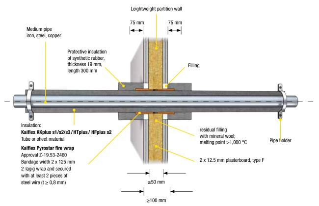
Kaiflex Pyrostar is fed through the metal stand wall at a width of at least  $2 \times 125$  mm and applied to the continuous insulation in two layers. The fire wrap must be placed to leave approx. 45 mm in the component.
