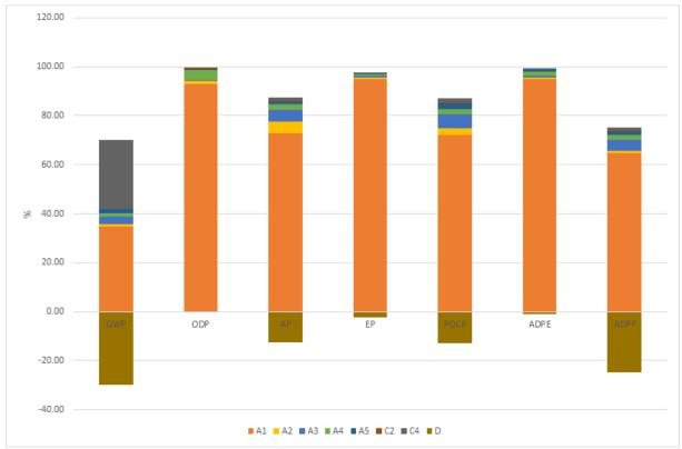
All seven environmental impact categories are dominated by module A1 raw material supply. The production of the blowing agent and the base material are the largest contributors. For the global warming potential, the incineration of the product in module C4 is another major source of greenhouse gas emissions.
