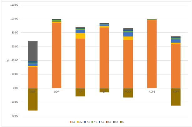
Most environmental impact categories are dominated by module A1 raw material supply. The production of the blowing agent is the largest contributors. For the global warming potential, the incineration of the product in module C4 is another major source of greenhouse gas emissions.
